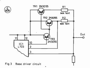
units containing the basic circuit, plus a built-in reference voltage and means of closing down the whole system if the current drawn by the load exceeds a preset amount. All this is furnished in the IC type L723 which is available in several variations from most of the major manufacturers; it is, in fact, an industry standard in the same way as the 741 is . Fig. 1 gives the circuit for using this device and the following notes will explain the various functions of the device.
