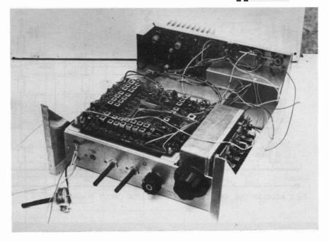
board that we have to build before we start is an oscillator unit that can provide a signal for each band we intend to cover. This will mix with the VFO to produce the required local oscillator signal for the transceiver mixer; this mixing of the two signals is done on the '707 RF board and the necessary filters are switched with the signal frequency circuits.
