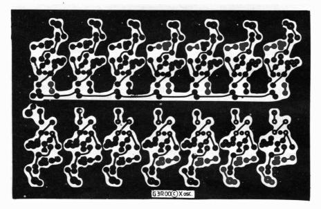
Fig. 4. Oscillator PCB foil
