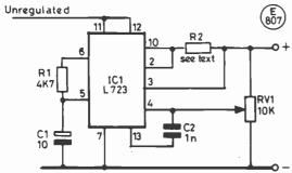
Fig. 1 Basic regulator with current limit
