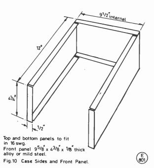
generally making a mess!) They charge a very fair price for a very high standard of workmanship and will make to order in either 16 or 18 swg aluminium. Finding a source of the 1/8 inch alloy for the front panel can be difficult but mild steel can be used with very little extra work.
