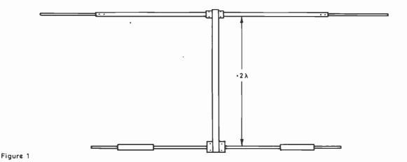
the *parasitic elements* in wet weather could seriously impair both gain and F/B ratio, and with the radiation resistance falling to some 18-20 ohms with close spacing, the losses in the radiator alone could amount to 30 per cent of the transmitter power (ignoring any additional losses in the parasitic elements!).
