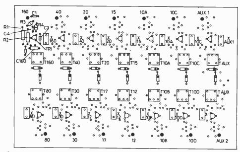
Components shown for 160M only. Repeat for other channels Terminal pin
