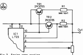
Fig. 2 Series pass section
