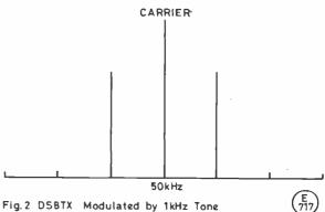
Fig. 2 DSBTX Modulated by 1kHz Tone
