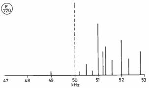
Fig. 5 Output spectra of SSB reduced carrier Tx.
