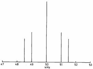
Fig.3 Modulation frequency of 1 & 1.5 kHz 1.5kHz amplitude less than 1kHz modulation
