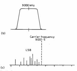
Fig. 10 Spectra after passing DSB signal through crystal filter to produce Lower Sideband Signal with Carrier frequency of 9001-5kHz.
