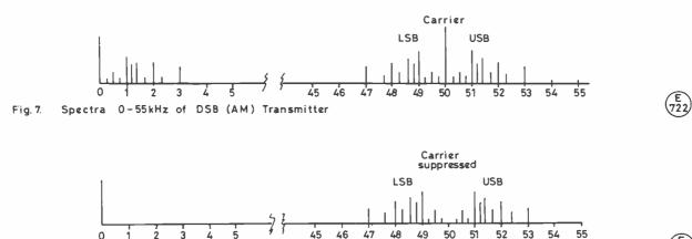
Fig. 8. Spectra 0-55kHz of DSB Suppressed Carrier Transmitter using Double Balanced Modulator
