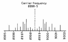
(a) DSB suppressed carrier from double balanced mod.
