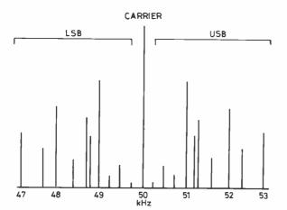
Fig.1 Double Sideband Amplitude Modulated Transmitter Typical Speech Spectrum
