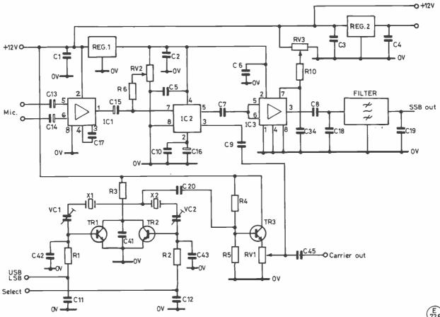
Fig. 11(a) Simple Sideband Exciter Circuit Diagram.
