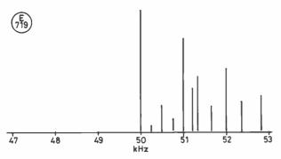
Fig. 4 Output spectra of Single Sideband Full Carrier.
