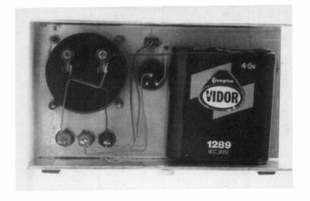
Inside view of the Ohm-meter, showing wiring
