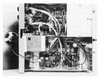
Under chassis showing (top) oscillator/mixer/bandpass assembly with switched low pass filters within shielded compartment on right, (bottom) Rx control assembly, and (middle left) the VFO box.
