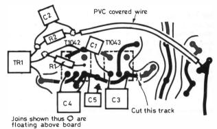
(b) Modifications and component additions to include amplifier to filter
