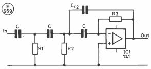
Fig. 4 HIGH PASS FILTER CIRCUIT
