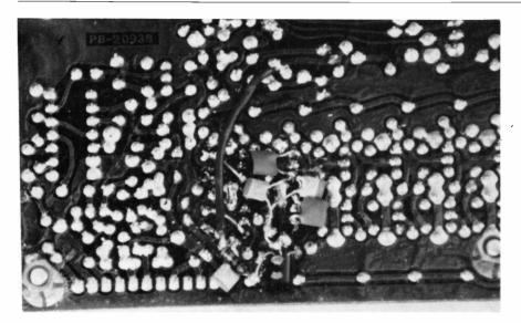
'Birdsnest' style amplifier on base of 'local' filter. See also Fig. 2(a) and 2(b).
