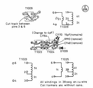
Fig. 3 RF PCB LAYOUTS IN VICINITY OF T1009 AND T1023 / T1024 AND REPLACEMENT COIL DETAILS
