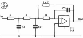
Fig. 3 LOW PASS FILTER CIRCUIT
