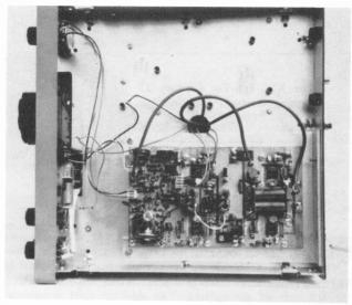
Above chassis view showing (top) area for keyer and calibrator mounting and (bottom) final amplifier assembly.
