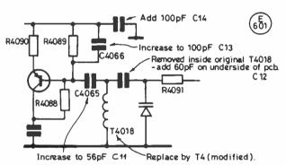
Fig. 4 ALTERATIONS TO THE VOLTAGE CONTROLLED OSC.(PLL.PCB)
