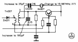
Fig. 3 ALTERATIONS TO CONVERSION OSCILLATOR (PLL PCB)
