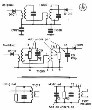
Fig. 2 RF STAGE TRANSFORMER CIRCUITS (Original and mod'd.)
