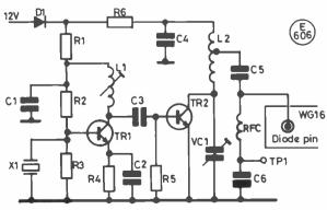
Fig. 3 CIRCUIT FOR AN ALTERNATIVE DRIVE UNIT
