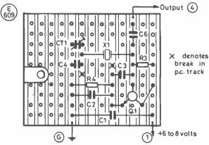
Fig.3 CRYSTAL OSCILLATOR COMPONENT LAYOUT
