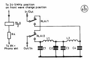
Fig. 6 LPF CIRCUIT DIAGRAM
