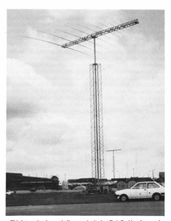
This interesting log-periodic array is sited at R.A.F. Alconbury and would appear to cover 12-30 MHz, the longest element being in the order of 40 feet or so. The photograph was taken by Peter Waters of Waters and Stanton Electronics during a recent air display there, and we wonder if his firm could supply a rotator for it!
