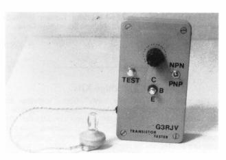
The completed transistor checker.
