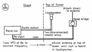
Fig.5 System used by N4AR to tune antenna with a Noise Bridge attached to antenna at the top of Tower.
