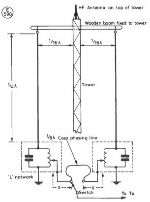
X = any length of coax but must be same length each side. See text re velocity factor of coax of  $1/8\lambda$  Phasing line. 'L' network requires a high 'C' (about 1000 pF) and a low 'L' as the impedance of verticals is approximately 32 ohms.
