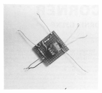
Layout of the transistor checker on Veroboard.
