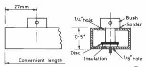
Fig. 2 Details of Diode mounting
