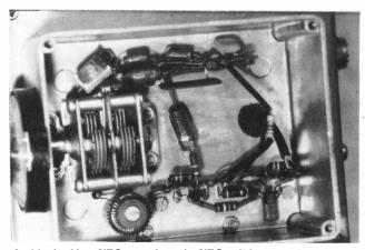
Inside the 80m. VFO: note how the VFO coil is secured.
