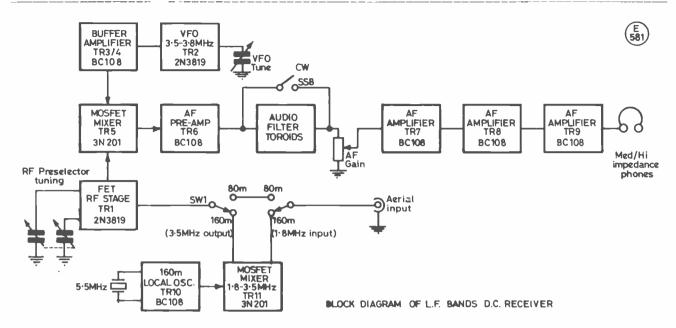
After amplification the RF signals are fed to a MOSFET double-gate mixer which was used primarily because of its conversion gain. Following the by now well known direct conversion techniques the resultant audio from the drain of the mixer is passed through an RF filter circuit to an audio pre-amp transistor and then *via* the CW filter to the audio gain control.
