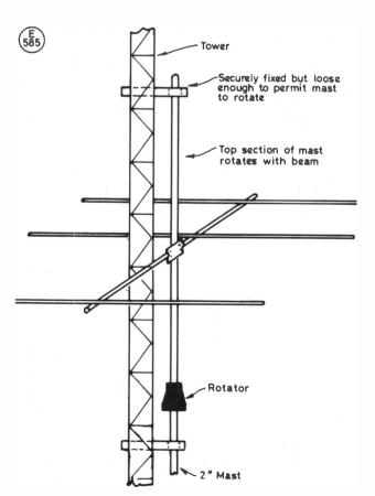
Fig. 4. System used by NAAR to permit a number of Yagi's to be mounted on the same tower and rotated independently of each other. They can only be rotated through 180° instead of 360°
