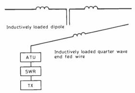
Fig.4 Suggested "loading points" for 2 types of inductively loaded antenna
