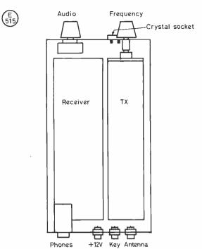
Fig.3. JLD TRANSCEIVER LAYOUT (Approx. half full size).
