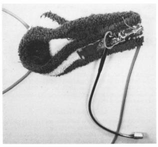
Showing method of fixing the boom to the headband.
