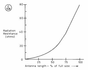
Fig. 5. Radiation Resistance of shortened dipole antennae. (Note: Figures do not include reactance)
