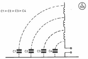
Fig. 3 Capacitance to earth at various points on a vertical antenna.
