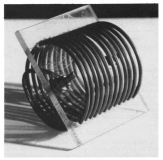
Fig. 8. An air-wound coil supported by a perspex former.
