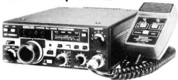
290D is the state of the art 2 meter mobile, it has 5 memories and VFO's to store your favourite repeaters and a priority channel to check your most important frequency automatically. Programmable offsets are included for odd repeater splits, tuning is 5KHz or 1KHz. The squelch on SSB silently scans for signals,
