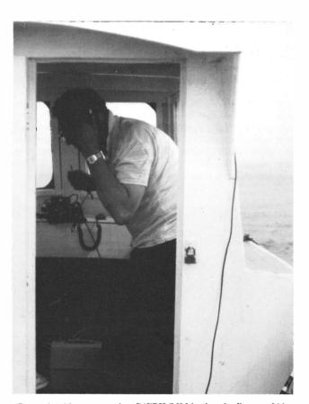
Bernard Atkinson operating G6EBH/MM in the wheelhouse of his diesel vessel *Prospect*. The transceiver is a Yaesu FT-290R with muTek front end. A Daiwa 30w amplifier is used with an HB9CV antenna for SSB and a  $\frac{7}{8}$ -wave vertical for FM/repeaters. The boat is 22ft. long and  $\frac{8}{6}$  beam with a  $\frac{12}{2}$  h.p. main engine and a  $\frac{7}{2}$  h.p. auxiliary. Listen for G6EBH/MM on summer weekends and sometimes on Wednesday afternoons from AO square on 2m.
