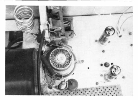
The 50 MHz PA. The mixer and driver are on the right, and the fan on the left.
