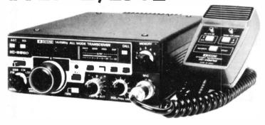
290D is the state of the art 2 meter mobile, it has 5 memories and VFO's to store your favourite repeaters and a priority channel to check your most important frequency automatically. Programmable offsets are included for odd repeater splits, tuning is 5KHz or 1KHz. The squelch on SSB silently scans for signals,
