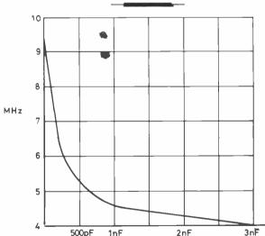
Fig. 3 Scale for extended range (560pF series capacitor).
