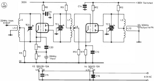
Fig.3 THE TRANSMIT BALANCED MIXER AND BUFFER AMPLIFIER
