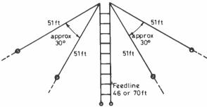
Fig. 4(c) Skeleton Cone Antenna (Get the lengths right but the angles can be compromised to fit in smaller spaces as inverted Vee configuration).
