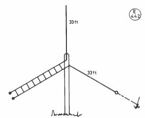
(a) Slanter for 40,20 and 15m (Also works well on 80m)
