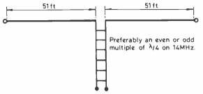
Fig. 4 (b) G5RV with open feeders
