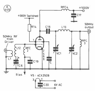
Fig. 4 50MHz PA (Note that the filament takes 6 volts rather than 6.3V. The capacitor 'C' is built into the SK620 valve socket).
