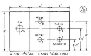
Fig. 8 Suggested layout of the transverter
