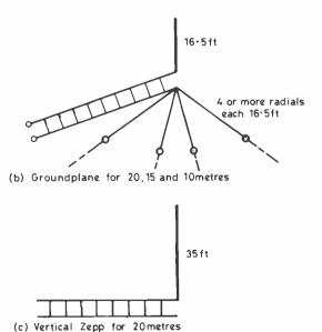
Fig. 5. SELECTION OF VERTICALS USING OPEN FEEDER
