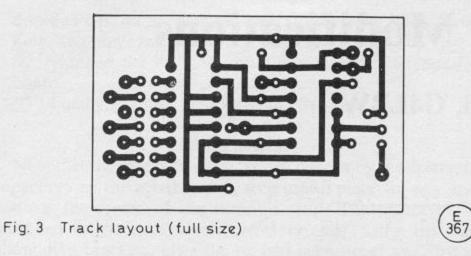
those nearest to the channel switch. Insert all of the resistors into the new PCB. Connect leads from the new PCB to the four veropins as marked, and then connect the digit leads to the outputs of the 74LS47. The supply can be taken from any 13.8ve and Ove source, as the board has its own 5ve regulator.
