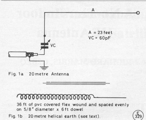
full length of dowel, and spaced approximately  $\frac{1}{2}$ " between turns. The connecting lead is four feet long, giving a total wire length of 36 feet, the whole device being suspended horizontally,
