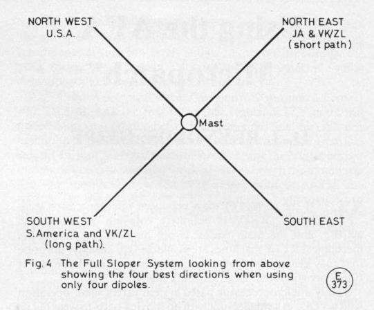
The sloper system had an advantage in that selection from one direction to another could be made immediately, whereas W2HCW had to wait for the rotator to go round.
