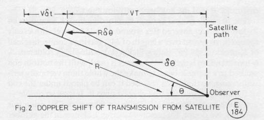
When the satellite is approaching the observer directly the Doppler shift in frequency, f, will be related to the transmission frequency, F, and the velocity of em-radiation, c, by:
