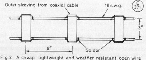
feeder suitable for use with the Extended Double Zepp or the G5RV array.
