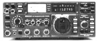
The IC-745's features include IF shift, 16 programmable memories with lithium battery back-up, passband tuning, a noise blanker both wide and narrow, threshold level control, notch filter, receive audio tone control and an all mode squelch. Also available is a front end switchable receiver preamp providing 12dB gain. RIT has a  $\pm$ 1KHz range.
