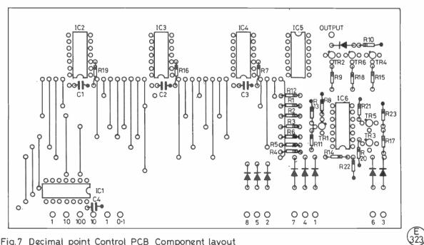
Fig.7 Decimal point Control PCB Component layout
