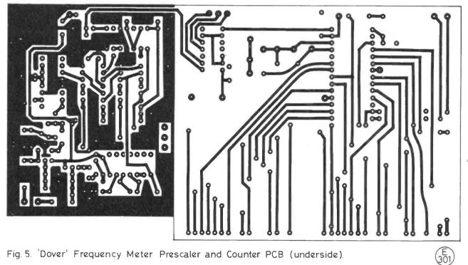
Fig. 5. 'Dover' Frequency Meter Prescaler and Counter PCB (underside).
