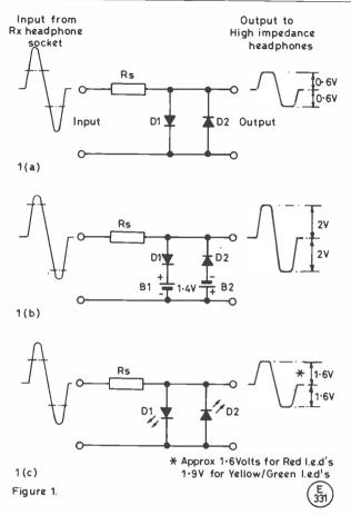
Fig. 1. (a), principle of operation of a shunt diode clipper/limiter circuit for connection between headphones and a receiver output; (b), reverse biasing of the diodes to increase the clipping threshold by the battery voltage; (c), using LED's as clipping diodes to take advantage of their higher forward conducting voltage — approximately 1.6v for Red LED's, and 1.9v for Green and Yellow ones.
