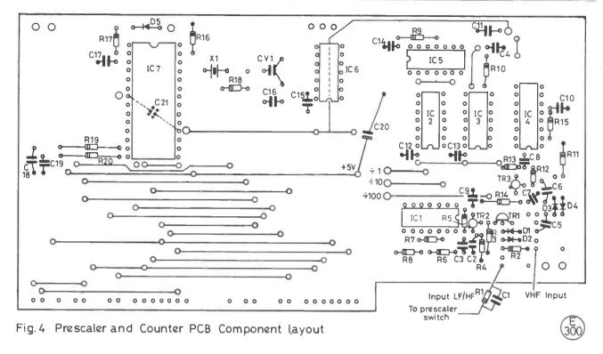
listed, firstly the gate period followed by the prescaler division ratio. As an example, if the switches are in the 0.1s gate period and the prescaler is in divide-by-100, group B decimal points are required and the decimal points associated with digits 1, 4 and 7 are illuminated.
