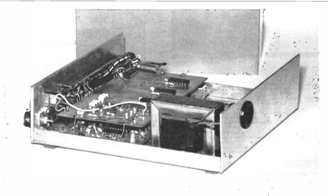
An inside view of the "Dover", showing both PCB's and transformer in position.
