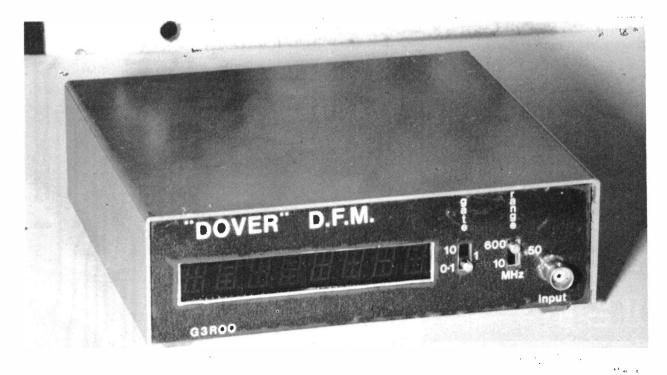
Front view of a completed "Dover" digital frequency meter.
