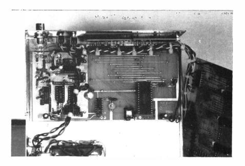
Showing the prescaler/counter PCB with decimal point control PCB removed (at right).
