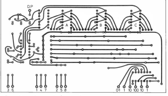
Fig.9 Decimal point Control PCB (underside)
