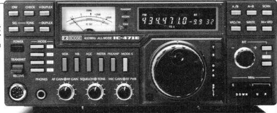
The IC-471E is the most advanced 430 MHz transceiver available today, it covers the spectrum from 430-440MHz with FM, SSB, or CW using the most advanced 10Hz PLL system. The IC-471E is suitable for simplex, repeater operation, moonbounce or satellite work, and has features found on no other transceiver.
