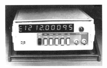
The Digimax Model D1200, shown above, is a compact, high-stability 50 Hz to 1.2 GHz frequency counter with several advanced features. The 0.1 p.p.m. 10 MHz oven is of special low current consumption design, and a built-in audio multiplier allows resolutions of 0.001 Hz to be achieved; operation is mains/battery. For full details contact Aspen Electronics Ltd., 2 Kildare Close, Eastcote, Ruislip, Middlesex HA4 9UR. (Tel: 01-868 1188, Telex: 8812727).
