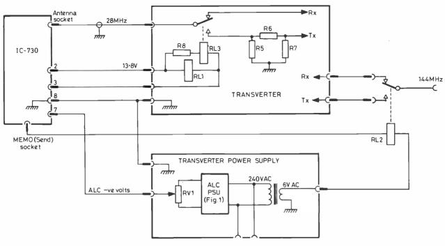
Fig. 2 TRANSCEIVER, TRANSVERTER AND POWER SUPPLY INTERCONNECTIONS The figures on the IC-730 diagram are the pin numbers on the accessory socket. An internal modification has to be made in the IC-730 to the "MEMO" socket (see text).
