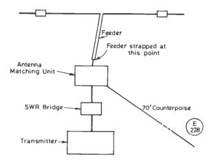
Fig.6 THE 4-BAND TRAPPED DIPOLE OPERATING ON 3-5MHz
