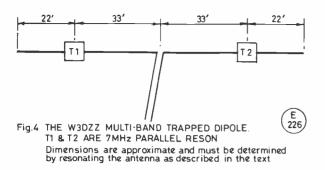
traps (*i.e.* 32ft. each side of the feeder) and approximately 22ft. for the outer sections, giving an overall length of around 108ft. this is depicted in Fig. 4. The lengths of the inner sections must be adjusted *first* to resonate the antenna at 7 MHz and *then* the outer sections are adjusted to establish resonance at 3.5 MHz.
