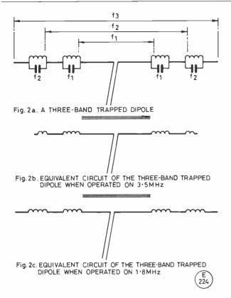
and 3-band dipoles discussed above, we saw that the traps acted as inductances when subjected to RF below their resonant frequencies, *i.e.* they behave as capacitors when subjected to higher frequencies. Fig. 3 shows traps in such a situation. The significance of this fact will become clear when we look at specific antenna types, which we will now do, and put the antennas in separate groups.
