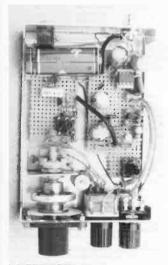
An inside view of the Mini-Monitor receiver, showing the VFO board behind the slow-motion drive assembly, with the main board behind RV1 and VC2. photo: Jo-Anna
