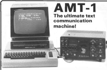
The LC.S AMT-1 AMTOR/RTTY/ASCII/CW Terminal Unit is extremely powerful in its own right, but combine it with a Commodore 64 computer and our new split screen program and it forms probably the ultimate amateur radio data communication system. Designed to get any home computer or ASCII terminal on the air with error-correcting data transmission with minimal difficulty, the AMT-1 is
