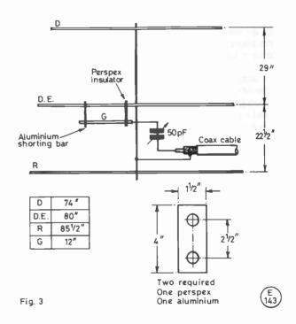
The beam can be set up by adjustment of the position of the shorting bar and tuning the variable capacitor whilst observing the wavemeter used as a RF field strength meter, simply tuning for maximum RF, or by using a VSWR meter if one is available.
