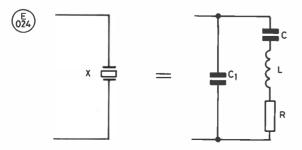
Fig.1 EQUIVALENT CIRCUIT OF A QUARTZ CRYSTAL
