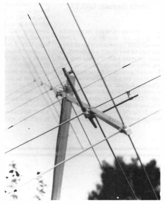
Fig. 1. General view from the rear of the MET Antenna type 144-6X. The mast-to-boom clamp is ingeniously designed to offer either a vertical and horizontal configuration, or an "X" or 45° one as depicted here.
