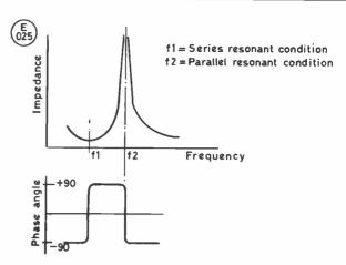
Fig. 2 GRAPHS OF IMPEDANCE AND PHASE V FREQUENCY
