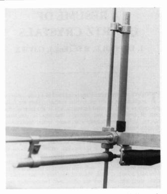
Fig. 3. Another close-up of the driven elements. A threaded brass rod is soldered to the N-socket, as supplied; the plastic boot is pushed onto the rod before screwing on the aluminium Gamma match rod. The boom is 19mm. square tube in two parts joined at elements no. 3; the driven elements are 6mm. diameter and the parasitic ones are 5mm.
