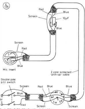
Fig.1 POINT-TO-POINT WIRING DIAGRAM
