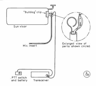
Fig. 2 GENERAL LAYOUT AND CONSTRUCTIONAL DETAILS.
