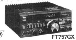
Frequency range 160-10m Tx general coverage Rx. 10 Hz VFO steps and 500 KHz band steps. Modes, USB, LSB, CW, AM, FM all as standard.
