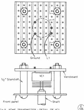
Fig. 5 ACME TRANSMITTER - DETAIL OF VC1
