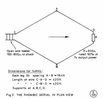
Fig. 3. The Rhombic is the 'Rolls-Royce' of aerials but needs much real-estate. This is a practical compromise design which should be able to yield 10-12dB gain in the preferred direction on 14/21/28 MHz, and be usable with some gain on 7 MHz. Refer to standard texts - *e.g.* ARRL "Antenna Book" – for deeper discussion.
