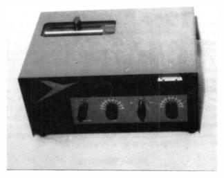
Fig. 3. An exterior view of the ATU showing the sliding link control on the top of the cabinet.
