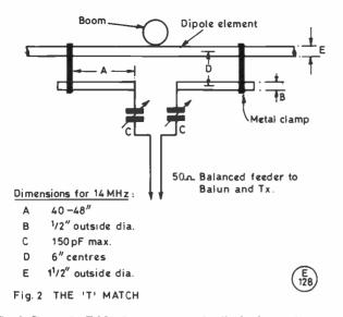
Fig. 2. Shows the T-Match system; note the dipole element is not split at the centre – this is known as 'plumber's delight' construction and is best for strength. The dimensions shown are approximate and would serve as a useful starting-point. In the absence of the capacitors, dimension 'A' would be different. The two capacitors must be adjusted 'in step' to maintain balance.
