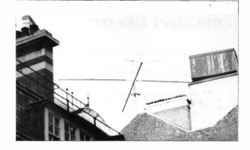
Nigerian High Commission: Communications to Lagos from the Nigerian High Commission in Northumberland Avenue are assured by means of this horizontal wire beam which is squeezed in between the chimney stacks.
