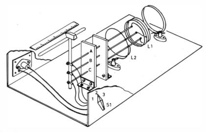
Fig. 1 MECHANICAL DETAILS OF THE VARIABLE LINK
