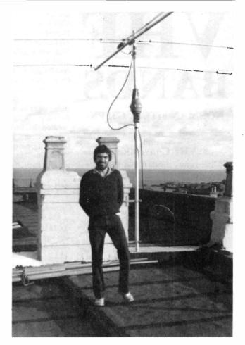
Ian, GW3WVG, with the triband beam on the roof of the hotel. The clear take-off to the north over the sea is in the background. LF antennas were supported by a 24-ft. pole lashed to another chimney stack.
