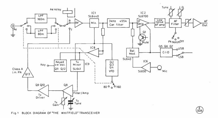
reduce any loss of gain in the receiver section. Plessey SL1600 devices would be used in the SSB generator, but Vogad (voice operated gain adjusting device) would not be employed on the grounds of cost. Actually, I rather doubt the value of Vogad in amateur use, but in commercial applications it is superb.
