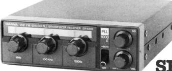
Now from Daiwa, a new 2 metre monitor receiver. Using PLL synthesized circuitry, the SR1000E covers the entire amateur band in 5 KHz steps. It provides for today's amateur a small convenient means of monitoring activity on the busy 2 metre band. Compact and supplied with earphone, mounting bracket, the SR1000 provides for you mobile or fixed your contact with the 2 metre band.
