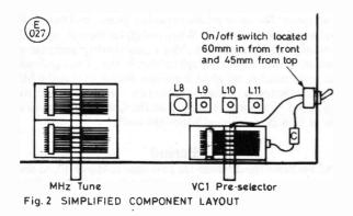
reception of *Radio 4* a slight adjustment to L11 may be found to be necessary if VC1 does not provide enough gain.
