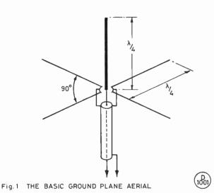
The horizontal radials act as an artificial earth or ground plane allowing the aerial to be mounted at any convenient height. Fed with a short run of good quality coaxial cable, this arrangement will normally radiate efficiently without resorting to lengthy tuning and matching procedures. Element lengths are not extremely critical and can be cut to: length = (234/f MHz)ft.
