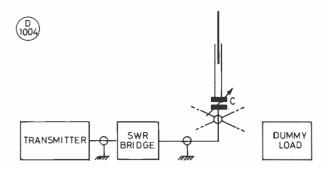
Fig.4 CONNECTIONS FOR THE TUNING & ADJUSTMENT OF AERIAL
