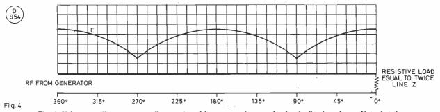
Fig. 4. Voltage standing waves on a line terminated in a pure resistance of twice the line impedance. Note that the minimum voltage points are at the same position as in Fig. 1, but the magnitude does not go to zero, nor is the maximum voltage as high.
