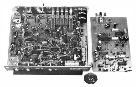
Fig. 2. View of the FL3 from the rear, with the automatic notch filter board detached. The sockets on the rear panel, from left to right are, Input, Tape output, 8-20v. DC supply and Output.
