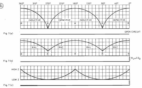
Fig. 7. Plots of reactance, resistance plus reactance and impedance on a line—see text.
