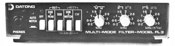
Fig. 1. Front view of the Datong FL3 Multi-mode Audio Filter, showing the neat front panel layout. The overall size is 184mm. wide, 44mm. high and 153mm. deep, the wrap-around case being anodised aluminium. The front panel is matt black with white and yellow legends.
