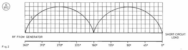
Fig. 2. Voltage standing waves on transmission line terminated in a short circuit—note that the minimum voltage points are more sharply defined than the maximum points.
