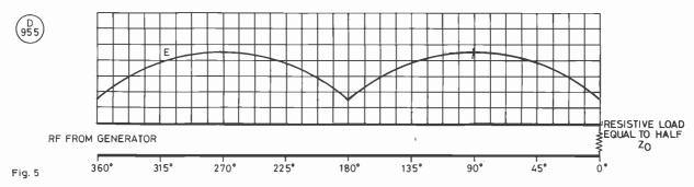
Fig. 5. Voltage standing wave on a transmission line terminated in a pure resistance of half the impedance of the line. The position of minimum voltage points correspond with those of Fig. 2, differing only in magnitude.
