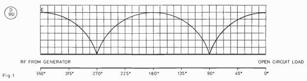
Fig. 1. Voltage standing waves on transmission line terminated in an open circuit, Note that the position of minimum voltage points is more easily established.
