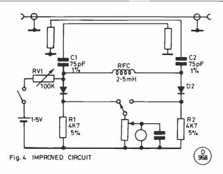
directions, suggesting good matching in the coupling and rectifier circuits. Further checking with a series of known resistors gave SWR readings in good agreement with their measured values, as did a dummy load the impedance of which (as indicated by a noise bridge) varies from 50 ohms at 3.5 MHz to 85 ohms at 30 MHz.
