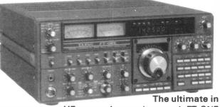
HF transceivers - the superb FT-ONE provides continuous RX coverage of 150KHz-30MHz plus all nine amateur bands (160 thru 10m). All-mode operation LSB, USB, CW, FSK, AM, \*FM • 10 VFO system • FULL break-in on CW • audio peak filter • notch filter • variable bandwidth and IF shift • keyboard scanning and entry • RX dynamic range over 95dB! and NO band switch!!!
