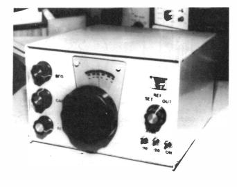
Above and below, a G3RJV 20-metre Transceiver in a two-piece case, with home-made scale assembly and epicyclic slow-motion drive as described in this series.
