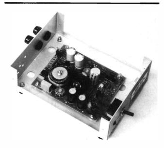
A new product from *Davtrend Ltd.* is the DRAE 24V/12V Switched Mode Convertor. This neat and compact power supply unit is ideally suited to communications applications where low noise and full protection are required. Current price of the 6 amp. version is £39.95 inc. VAT (a 10 amp. version is also available), and full technical specifications will be sent on request by the designers and manufacturers, Davtrend Ltd., 89 Kimbolton Road, Portsmouth, Hants. PO3 6DA. (Tel: 0705-816237).
