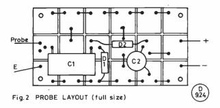
be soldered; tin the copper first then solder the lead to the copper square. Several shorting links will be noticed on the layout in Fig. 2. These, if they are not wires to join various squares in the circuit, are links to join up the spare copper square to form an earth mat around the circuit. So the bottom row of squares, which forms the earth side of the circuit, and the top row of squares are all joined in line.
