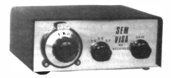
S.E.M. announce the availability of the 'Visa', their new receiver for the amateur. Priced at £39.00, it is intended as a receiver for the beginner or as an additional shack Rx. Measuring only  $2\frac{1}{2}$  x 6 x 3 inches, coverage is 3.5 to 3.8 MHz (80 metres in three 100 kHz bands), audio output 2 watts, selectivity  $\pm 2$  kHz, and sensitivity 1  $\mu$ V. Full specifications are obtainable from S.E.M., Union Mills, Isle of Man.
