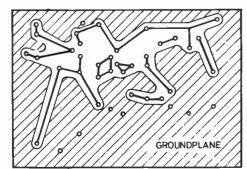
Fig. 2 VFO PCB. Double sided board. Top side used as earth groundplane, shorted to lower groundplane at various points
