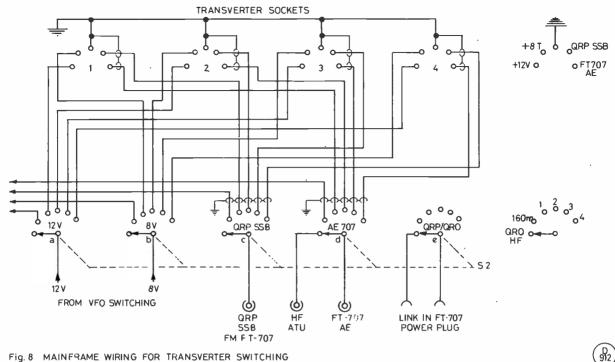
Fig. 8 MAINFRAME WIRING FOR TRANSVERTER SWITCHING
