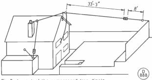
Fig.7 Layout of the compressed trap dipole
