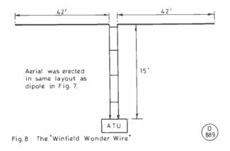
The aerial is still in use at the time of writing, and has been used with ATUs having both balanced and unbalanced outputs, although in the latter case, one leg of the aerial would have been acting simply as a counterpoise. It was mentioned earlier that initial tests seemed to indicate that signals on 80m. were down slightly compared to the 110-ft. version, but this may well have been Murphy up to his tricks, since the aerial has since proved
