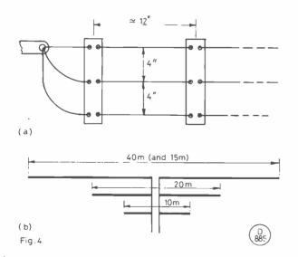
Fig. 4*a*. Construction of a three-band parallel dipole aerial; the spacers are made of strips of plastic. Fig. 4*b* shows a four-band dipole, using three parallel wires. Although the 40m. dipole will also be resonant on 15m., the SWR will be about 1.7:1 so solid-state rigs may need an ATU; the SWR is due to the higher feed impedance on 15m.
