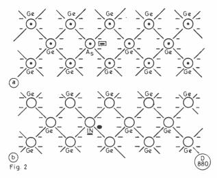
Fig. 2. Here we have introduced avery small impurity (as little as 1 part in  $10^{11}$  is significant). At (a) the impurity is arsenic, which has a valency of five; hence we have one electron surplus as shown. At (b) the impurity is indium, which is trivalent, resulting in an incomplete bond due to the 'missing' electron, shown as a hole in the drawing.
