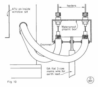
Fig. 10. Detail of the feeder junction at the window frame. The box used by the author was a 'plastic imitation' of a diecast box; the mains cable used for the earth lead has all three cores in parallel, and is connected to an earth rod at the foot of the wall.
