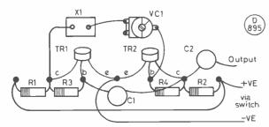
Fig. 4 CRYSTAL CALIBRATOR LAYOUT
