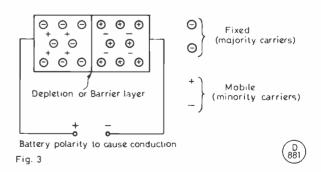
Fig. 3. Here a piece of germanium is doped to give P- and N-type areas, resulting in a depletion layer at the junction, where the mobile carriers from each side cancel, leaving a 'no-man's land' between the areas (in the absence of external effects). Connecting a battery as shown will cause conduction; if the battery is reversed, no current flows.
