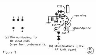
input coil TO8, and remove its can by alternately unsoldering each of the two lugs and "walking" the can upwards. This method will not work for the coil itself, which has 5 pins (Fig. 2a) and is easily damaged by excessive heat. Instead, carefully cut and shape a piece of aluminium so that it just fits within the rectangular area between the coil pins. Heat the aluminium with a soldering iron, and all 5 pins will be unsoldered at once, allowing TO8 to drop out undamaged.
