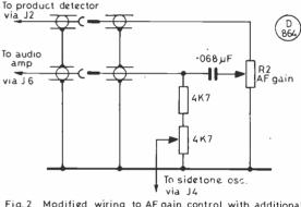
ig. 2 Modified wiring to AF gain control with additional components to provide preset sidetone level facility.
