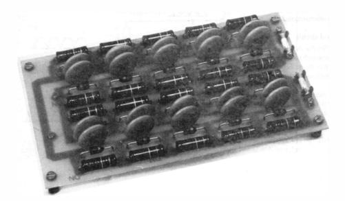
The rectifier stack used in the prototypes; note the equalising resistors and capacitors. The latter are rather vocal when thyristor drive is in use! Note also the "anti-Murphy" fuses in clips at one end of the board. Correct fusing, for semiconductors is most important, and is discussed in the text.
