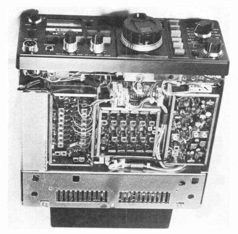
Bottom view. The boards from left to right are the Bandpass Filter Unit, Premix Unit and PLL Unit, shown here with the clip-on screening covers removed. The screw for altering the "feel" of the tuning knob can be seen on the bottom below the knob and can be accessed through a hole in the bottom cover of the case.
