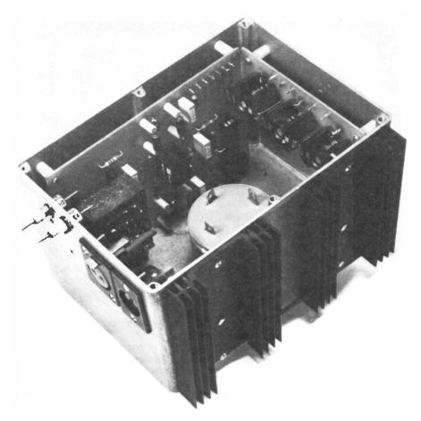
General view of the SCR stack box. The heatsinks carrying the main thyristors are rated at 4 degrees C per watt, and TO220-style devices were used in this particular version. Note the two vertical PCBs carrying the main electronics and the inductors used for dV/dT protection and RFI suppression. The photograph shows one of the engineering prototypes before wiring was complete.
