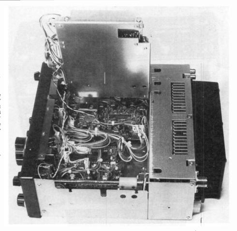
Underneath the Main Unit p.c.b. are the Logic Unit board, nearest the bottom of the picture; and the Second IF Unit p.c.b. with spaces for the optional SSB Passband Tuning and Narrow CW filters (added later) to the right rear. The Second Local Oscillator board is under the screening box at the left.
