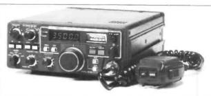
TR9500 The TR9500, a 70cm multimode mobile giving SSB, FM and CW operation in a compact rig based on the phenomenally successful 2 metre 9000. Combining the convenience of FM with the "DX ability" of SSB on the 70cm band this is the rig all discerning VHF and UHF amateurs have been waiting for.
