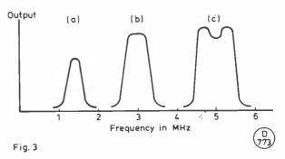
A simple representation of the change in selectivity over the frequency range of the pre-selector due to the increase of coupling between the tuned circuits as the frequency is increased.
