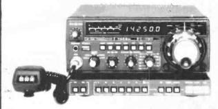
The definitive HF mobile rig, digital, variable IF bandwidth, 100 watts PEP SSB. AM, CW (pictured here with 12 channel memory VFO). Latest bands
