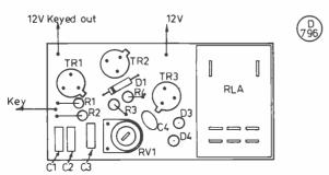
Fig. 6 CHANGEOVER CIRCUIT BOARD (actual size).
