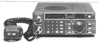
TR7800 Trio's remarkable TR7800 2-metre FM mobile transceiver provides all the features you could desire for maximum operating enjoyment. Frequency selection is easier then ever, and the rig incorporates new memory development for repeater shift, priority, and scan. The TR7800 by Trio, the only FM mobile.
