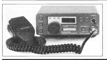
The compact DFC230 Digital Frequency Controller provides maximum efficiency and flexibility for mobile and fixed operation by combining a 20 Hz step digital VFO with 4 memories. ● 20 Hz step digital VFO: ● Four memories: Frequency can be transferred from VFO to memory or from memory to VFO. ● Frequency can be transferred from VPO to memory of normal memory to VPO.
