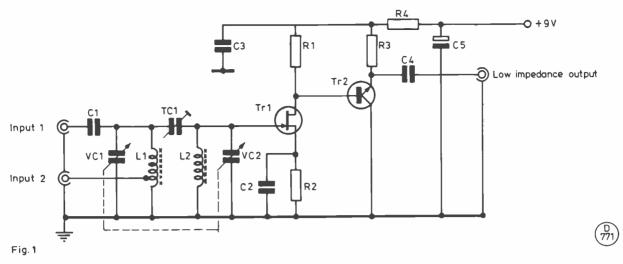
The circuit of the pre-selector as built to cover a frequency range of 1.4 to 5.00 MHz. Other frequencies can be covered by proper choice of L1 and L2.
