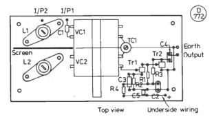
Fig. 2 The component layout for the pre-selector. Components are assembled on a piece of Veroboard 130mm x 65mm.
