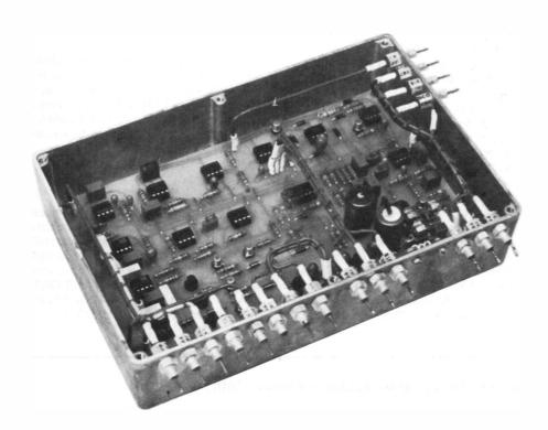
A general view of the control unit — note the feedthrough capacitors used to take connections into and out of the box. The unit contains all the control electronics, trip sense amplifiers, low-voltage regulators for the op-amp supplies and everything necessary to drive the SCR stack. It is basically Figs. 2, 3, 4 and 7.
