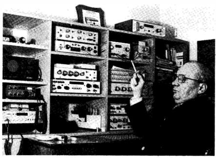
The shack of Mirko Voznjak, YU1AD, in Belgrade. On the extreme left, from the bottom, is an Astro 200 transceiver with SWR bridge, a Trio TR-9000 2m. multimode, and a Trio Monitorscope. The vacant space at the top is for a Mirage 80 amplifier. The rest of the gear is purpose-built test equipment for engineering and development work. Mirko usually spends three months each year in England when he works as a service engineer for *Radio Shack Ltd*. in London.
