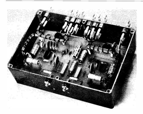
A general view inside the box. The BZY93C75R Zener diodes are bolted directly to the box, with holes for adjustment of the presets directly below them. The 62K/2W resistors are mounted on ceramic stand-offs above the board, and the VDR's across the output of one channel can be seen below the left-hand cableform.
