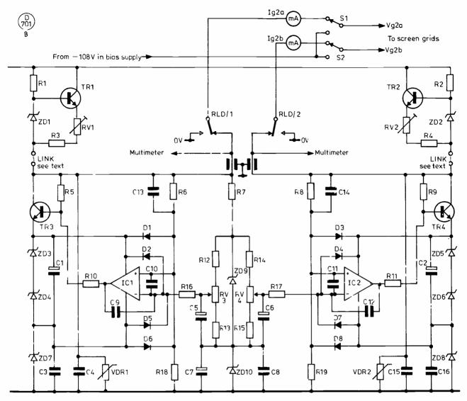
Fig 4 SCREEN VOLTAGE SUPPLY UNIT FOR HIGH PERFORMANCE POWER SUPPLY AND CONTROL UNIT
