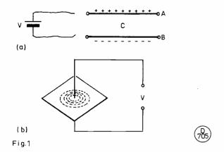
Fig. 1a. A voltage, V, has been applied between the upper wire, A, and the lower wire, B. If the voltage is raised enough, there will be a flashover through C (the dielectric). In Fig. 1b, the wire passes through a stout piece of paper sprinkled with iron fillings, the current producing a magnetic field. See text.
