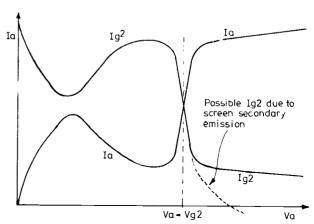
Fig. 2 ANODE AND SCREEN CURRENT CHARACTERISTICS FOR PRACTICAL TETRODE
