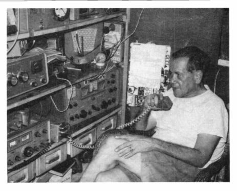
Derek Jeffries, VU2BEJ, is on the air regularly from his QTH in Bombay, and always pleased to QSO UK stations. The rig is an FL-DX400 Tx, HQ-180 Rx and SB-200 linear; antenna is a two-element 3-band quad on top of a 150-ft. high building. *Photo: G3ZXZ*
