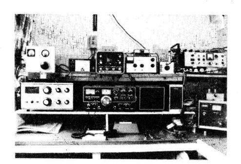
This tidy station belongs to A. F. (Bert) Bower, G3MKU, of Shepshed, Loughborough, and comprises a TS-520, a TL-911 linear and a Europa 'B'; for experimenting on 70cm. there is a U.450L Tx and a receive converter feeding a 9R-59DE Rx. Antennas consist of a 90-ft. long-wire for 80m., a Mosley TA-32 for 20-15-10m., an 8-ele Yagi for 2m., and a 9-ele for 70cm. On the ancillary front, there is a PM-2000 wattmeter, monitorscope, SWR bridge and home-brew Z-match.
