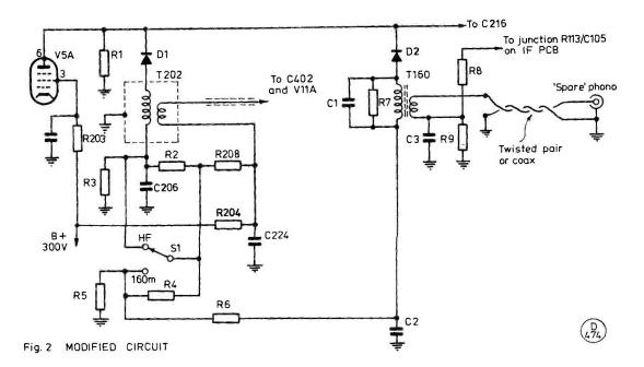
The bandwidth of the 160m. tuned circuit is designed to about 200 kHz (by the addition of R7) and so the circuit does not require peaking when the transceiver frequency is changed from one end of the band to the other. The output is taken to the 'spare' phono socket on the rear apron of the transceiver and a voltage for controlling the selection of the linear and pre-selector, derived by R8 and R9, is also carried by this socket.
