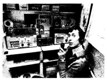
The station of well-known VHF operator Geoff Brown, GJ4ICD, from St. Saviour, Jersey, Left to right:  $2 \times 4C \times 250B$  2m. amplifier and power supply. Trio TS-700 (since replaced by a TS-770) with a Bird Type 43 power meter above, and a K2RIW 70cm. amplifier with PSU.
