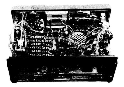
Fig. 1. View of the top from the rear. The six RF bandpass filters are the group of 32 canned coils. The three 455 kHz ceramic IF filters are grouped behind the main tuning mechanism, the plug just to the left being *Lowe Electronics*' alternative bandwidth selection (see text).
