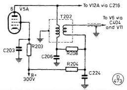
Fig.1 HW-101 SECOND MIXER INPUT/OUTPUT CCT.
