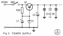
The transistor will require a heatsink. Capacitors C3 to C8 are IC power supply decoupling capacitors, and should be distributed over the board close to the IC's.
