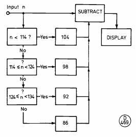
Fig.1 Logic flowchart of Digital Channel Display
