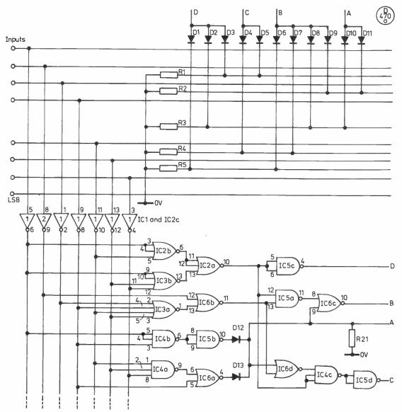
Fig. 2 DIGITAL CHANNEL DISPLAY CIRCUIT DIAGRAM
