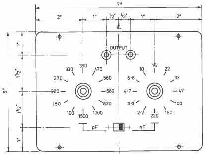
Fig. 1 FRONT VIEW OF CAPACITY BOX (Knobs omitted for clarity).
