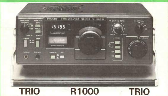
The R-1000 uses an advanced PLL system in an up-conversion scheme to a high (48MHz) first IF to remove any possibility of image responses. The receiver covers the entire frequency range from below 200kHz right up to 30MHz in 30 bands, each 1MHz wide. The bands are selected, not by ambiguous knob twiddling as in receivers using the Wadley loop but by a 30 position band switch which controls the PLL system.
