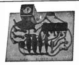
455 kHz FM Discriminator Amplifier. Limiting threshold 100uV. Amplitude modulation rejection 40dB. Audio output voltage at 1 kt.1 200-300mV frequency deviation + cr - 3 kHz. Price £5.00
