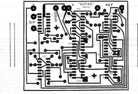
Fig. 4. Printed circuit layout of C-MOS keyer, showing foil side.
