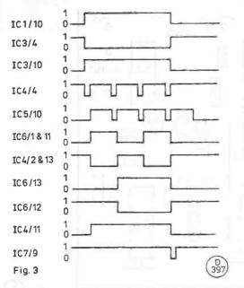
Fig. 3. Logic timing diagram for dash generation.
