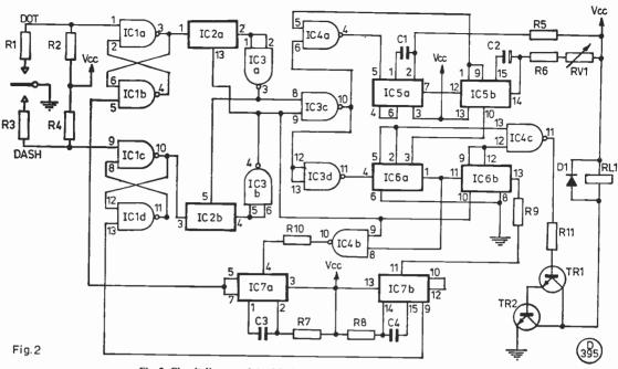
Fig. 2. Circuit diagram of the G3TAG C-MOS keyer. See also Figs. 2a and 2b.
