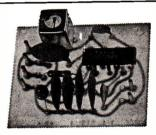
455 kHz FM Discriminator Amplifier. Limiting threshold 100uV. Amplitude modulation rejection 40dB. Audio output voltage at 1 kl. 200300mV frequency deviation + or -3 kHz. Price 45.00
