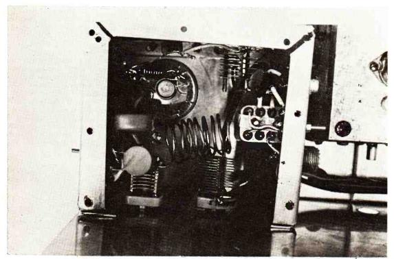
Looking into the PA compartment; placement of the various components can be clearly seen.
