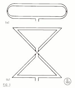
Construction of the XJK Antenna from a length of lighting flex: (a) the ends of two equal lengths joined to form a loop; (b) the joins cross over at the centre.
