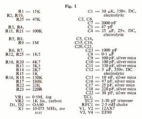
Note: All capacitors are disc ceramic, 1000v. DC working, unless otherwise stated.
