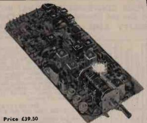
ARIO Mosfet receiver. 28-30 MHz Double conversion superhet. RF and amplifiers stages are gase protected mosfets for good sensitivity and low intermodulation. Noise limiter and squeich circuit. AM, SSB and CW reception. 12v. DC.
