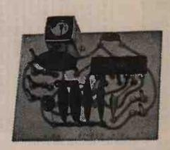
455 kHz FM Discriminator Amplifier. Limiting threshold 100uV, Amplitude modulation rejection 40dB. Audio output voltage at 1 kHz 200-300mV frequency deviation + or — 3 kHz. Price £5.00
