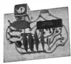
455 kHz FM Discriminator Amplifier. Limiting threshold 100uV. Amplitude models-tion rejection 40dB. Audio output veltage at I kHz 200-380mV frequency deviation - 3 kHz. Price £5.00
