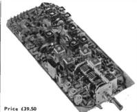
AR10 Mosfet receiver. 28-30 MHz Double conversion superhet. RF and amplifiers stages are gate pretexted mosfets for good sensitivity and low intermodulation. Noise limiter and squelch circuit. AM, SSB and CW reception. 12v. DC.
