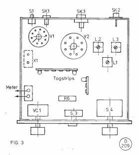
circuit to drive V2. The PA stage is conventional with cathode keying and there is no need even to buy a panel meter for the station testmeter can be made use of. All coils are hand wound—L1, L2 and L3 being made 'peakable' be means of VC1 which is protected against DC by C5. Switch S3 will enable 'Drive,' and PA current monitoring R (the meter shunt) being adjusted experimentally to permit, say, a 0-10mA meter to read 0-100mA f.s.d. in the anode position.
