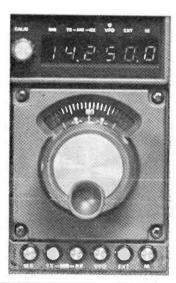
Offset tuning for either transmit or receive frequency allows precise zeroing in on that rate DX.
