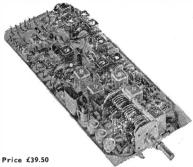
AR10 Moslet receiver. 28—30 MHz Double conversion superhet. RF and amplifiers stages are gate protected mosfets for good sensitivity and low intermodulation. Noise limiter and squelch circuit. AM. SSB and CW reception. 12v. DC.
