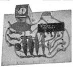
495 kHz FM Discriminator Amplifier, Limiting threshold 1004V. Amplitude modulation rejection 40d8. Audio output voltage at 1 kHz 200-390mV frequency deviation + or - 3 kHz. Price £5.00
