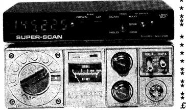
★ Scans 40 channels in 25 kHz steps from 145.000 when scan mode is selected. Locks out unwanted occupied channels
