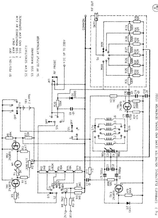
COMBINED ELECTRONIC VOLTMETER (EVM) AND SIGNAL GENERATOR (SSG) m
