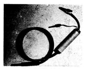
Fig. 4. The RF Diode Probe.
