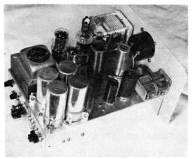
The home-built Top Band transverter made by Edgar Janes, G2FWA, and used as part of the gear operated by the Cheltenham Amateur Radio Association during MCC.
