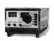
AR10 Mosfet receiver. 28-30 MHz Double con-version superhet. RF and amplifiers stages are gate protected mosfets for good sensitivity and low intermodulation. Noise limiter and squelch circuit. AM. SSB and CW reception. 12v. DC.
