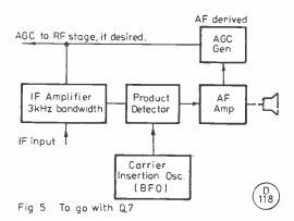
The front-end of an SSB receiver can be conventional and is not shown. IF signals are amplified in the selective stages before going to a mixer ("product-detector") stage. The AF output goes through an amplifier and AGC may be audio-derived as shown. Carrier re-insertion is by way of the BFO, which is set to be at the "carrier frequency" when the signal is correctly centred down the IF amplifier.
