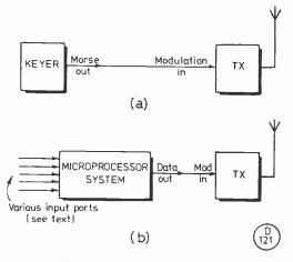
Fig. 1. (a) The present system used in beacons. (b) The "Microprocessor Controlled Beacon" as envisaged by G8KGV.
