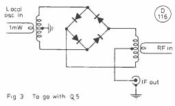
A good mixer circuit with few components. Note how the diodes are connected—not like a bridge rectifier! The diodes should be matched or, preferably, hot-carrier diodes. Note the high injection at the local oscillator input —this is important for best response and good overload characteristics. This mixer will have a few dB of insertion loss and should be preceded, above 144 MHz at least, by an RF stage.
