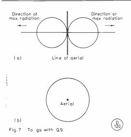
(a) Polar diagram of half-wave dipole, folded dipole, centre or end-fed Zeppelin aerials. This shows direction of radiation strongest at right-angles to the aerial. Angle of radiation upwards is a function of height of aerial. (*Note*: with Zeppelins some distortion due to feeder radiation is likely.) (*h*) Polar diagram of loaded vertical shows equal radiation all round.
