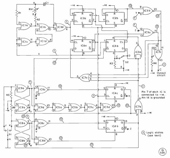
Fig. 3. Logic diagram of the Keyer.
