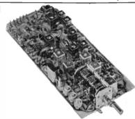
ARIO Mosfes receiver. 28-30 MHz Double conversion superhet. RF and amplifiers stages are gate protected mosfets for good sensitivity and low intermodulation. Noise limiter and squelch circuit. AM, SSB and CW reception. 12v. DC.
