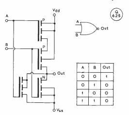
Fig. 1. Circuit diagram and truth table for a NOR gate.
