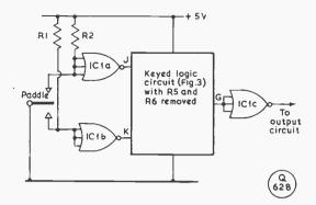
Fig. 5. Additional circuitry required when keying positive voltages.
