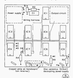
Fig. 6. The construction technique and layout used in the prototype.
