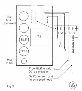
A five-way tag-board is mounted over the piercings disclosed by removal of the original modulation transformer from the TR1986 modulator unit; it picks up HT, LT and E lines from within the unit, and is fed with HT, LT and E from the existing transmitter. Pins 4 and 5 connect to Pin 6 on each of the (C4 valve sockets to pick up the output from the EL91 driver valve in the modulator unit. output then feeds the CO screen in the existing VHF transmitter.
