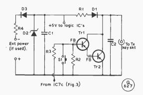
Fig. 4. Power supply and output circuit.
