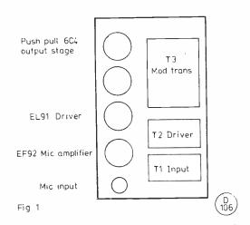
The TR1986 modulator chassis in plan view. To modify it for FM involves removal of transformers T1 and T3, and of the push-pull output valves. The output of the driver EL91 is then used to modulate the screen grid of the CO stage in an existing VHF transmitter.
