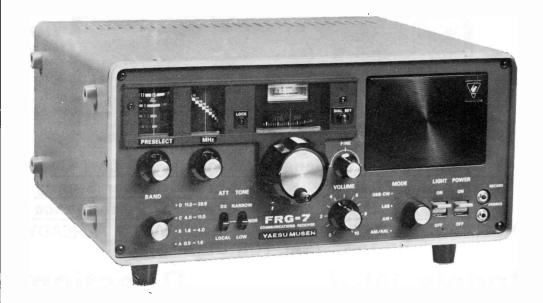
UNPRECEDENTED SENSITIVITY, SELECTIVITY, STABILITY AND DIAL CALIBRATION 0.5 kHz TO 29.9 MHz COVERAGE WITHOUT GAPS
