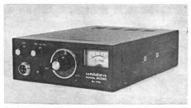
UNIDEN 2030. 144-146 MHz FM Transceiver. 12 channels. 12v. DC operation. 10 watt or 1 watt output. Antenna impedence 50 ohm. Complete with microphone and mounting bracket. Price £178-74
