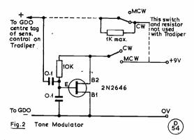
the dipper is a free running oscillator the frequency of which is inherently influenced by variations in supply voltage.
