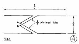
The problem now was to convey the signal from AB, where the impedance is 350 ohms balanced to the receiver input which is "50 ohms nominal" unbalanced. A 4-to-1 Balun seemed to be the obvious answer here, producing 87.5 ohms unbalanced, and an ATU would complete the task.
