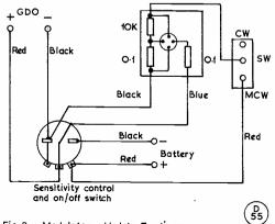
modulated signal on a receiver. If the level of the audio tone is adequate without the resistor, omit both it and the second pole of the switch.
