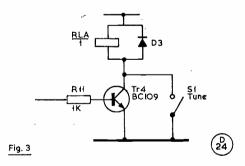
line was the positive side but in some of the newer transceivers it will be found that the keying line will be negative with respect to earth; in this case the earth should be connected to the collector and the keying line to the emitter. It is best to leave the collector and emitter connections floating so that the keyer can be used with any transmitter.
