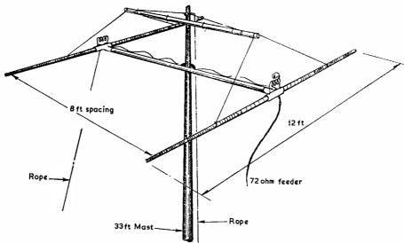
Fig. 1. Method of mounting MINI-ZL
