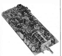
AR10 Mosfet receiver. 28–30 MHz Double conversion superhet. RF and amplifiers stages are gate protected mosfets for good sensitivity and low intermodulation. Noise limiter and squelch circuit. AH, SSB and CW reception. 12v. DC.
