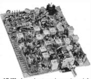
AT 222. A complete transmitter exciter unit for 144–146 MHz on AM or FM. VFO controlled or fixed channel operation. Complete with microphone pre-amp, speech processor including active audio filter. I watt output. FM. 25 watt AM. Output impedance 50–75 ohm adjustable. Frequency deviation 3–10 kHz adjustable.
