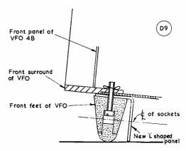
Fig. 2 METHOD OF FIXING TO VFO
