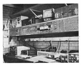
University of Surrey AMSAT-UK Telecommand Centre. The station runs entirely automatically, being computer programmed for a week at a time. (Fig. 1)
