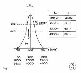
one tunes the receiver up in frequency the selectivity becomes worse and we cannot control it to the minimum bandwidth required for the signal. A receiver designed to receive only one frequency in the MF or LF bands could well be a "straight" set, but if we wish to tune over a band of frequencies we are in trouble. There is therefore a case for changing all signal frequencies received to one specific frequency which we can deal with properly, and this leads to the superheterodyne principle.
