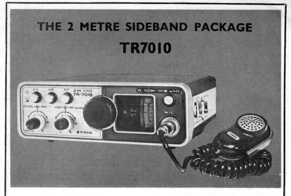
If your station is equipped for FM only, and you wonder where other 2 metre operators have gone when conditions are goodjust borrow a receiver and listen to the SSB around 144-3. DX contacts with continental stations are commonplace because of the sheer distance covering ability of SSB. With the freedom from channel restrictions and the ability to have multi-station QSO's with ease, SSB capability can add a new dimension to your amateur radio 2 metre operations.
