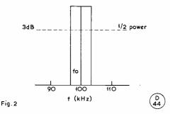
adjacent signal 3 kHz removed from  $f_0$  and thus out of band. If this signal strength is the same as our wanted signal it will pass through to the receiver output with only 6 dB attenuation, and thus cause interference. Note that both tuned circuits have the same selectivity figure, and it becomes apparent that this figure is not, in itself, adequate to judge a receiver performance in respect of both linearity of frequency response and protection against adjacent signal interference.
