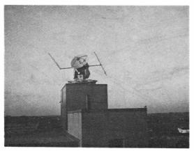
University of Surrey. The dish aerial and  $3\frac{1}{9}$ -ton tracking mount; the crossed polarised Yagis for 70 cm. and 2m. are on the left and right respectively. The dish is presently used on 10 GHz for colour TV experiments, and the whole array is on a 110ft. high tower. (Fig. 2)
