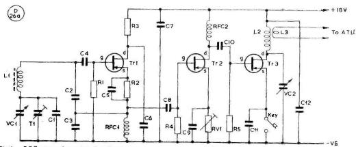
Fig. F.E.T. transmitter for Top Band.
