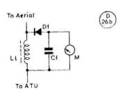
Fig. 2 Aerial tuning indicator for very low power tx.
