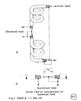
Wind a length of solid dielectric cable 16ft. 6in. long into a nine-turn coil, first making the centre as shown in "B" and covering with waterproof PVC tape; where the drawing shows "coaxial feed" a suitable coaxial connector should be fitted, to mate with the one on the feeder. Use RG58A/U or UK equivalent for 50-ohm impedance, RG59A/II or UK equivalent for 72-ohm impedance (solid-polythene dielectric).
