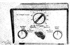
Mk. I MULTI TUNER. Designed and manufactured by us. 50 tunable switched positions for antenna lengths over 5 metres in the 2-30 MHz range. Five different circuits to give an excellent match between your receiver and antenna. Now in use in over 35 countries. Price £17.50. Including VAT and Postage.
