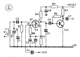
Fig.f Simple receiver adaptor circuit
