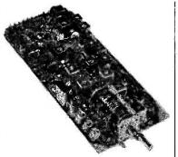
AR10 Mosfer receiver. 28–30 MHz Double conversion superhet. RF and amplifiers stages are gate protected mosfets for good sensitivity and low intermodulation. Noise limiter and squelch circuit. AM, SSB and CW reception. 12v. DC.
