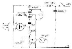
Fig. 2 Circuit for FET VHF Dipper.
