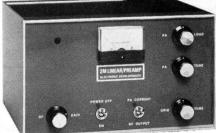
This Linear Amplifier has been developed by us to fill the need for a high power add-on unit for use mainly with low power SSB transceivers. The unit also contains a lcw-noise receiver preamplifier which is equipped with an RF gain control. Mains operated. Drive requirement: 5-20 watts. CW and SSB, 5 watts maximum AM & FM. P.A. 50% efficient. R.F. switched so no modification to transceiver is necessary.
