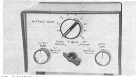
Mk. I MULTI TUNER. Designed and manufactured by us. 50 tunable switched positions for antenna lengths over 5 metres in the 2-30 MHz range. Five different circuits to give an excellent match between your receiver and antenna. Now in use in over 35 countries. Price £17.00. MK2 Multi-Tuner covering 550 KHz to 30 MHz. £23.00
