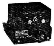
This 432 MHz Linear is operated in grounded grid configuration and exhibits a gain of typically 10dB. With a drive input of 5 watts its output power is in the order of 50 watts which is more than adequate for OSCAR 7. Power requirements are 6·3v. AC and H.T. 400–1000v. DC. Fitted with BNC connectors.
