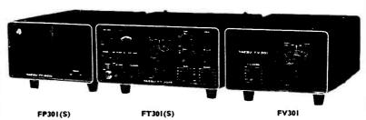
The transceiver employs a pre mix VFO and single conversion signal frequency IF (9 MHz) uses MOSFETS in the RF and mixer stages followed directly by a roofing filter for sensitivity coupled with dynamic range.
