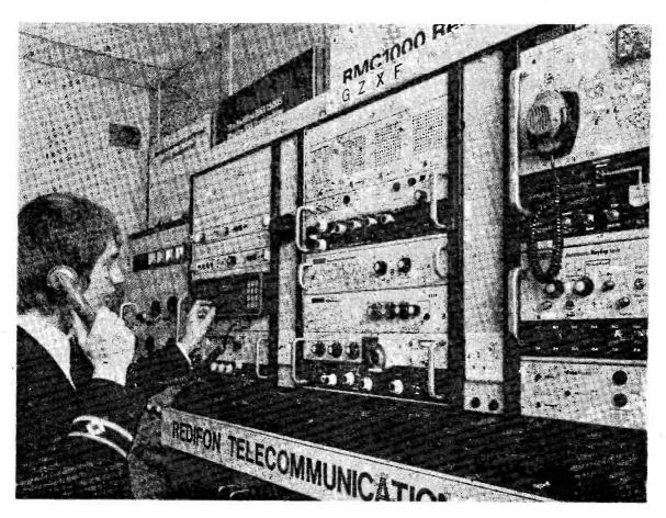
This marine radio console by Redifon Telecommunications is the Company's new mobile demonstration unit. The user is offered a greater choice of technically advanced modules, including the ship's main station on HF/MF, dual watch VHF radiophone and auto-alarm. The console complete is factory tested and has international type approval. It can be quickly fitted and the test callsign is GZXF on the marine bands.
