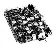
AT 222. A complete transmitter exciter unit for 144–146 MHz on AM or FM. VFO controlled or fixed channel operation. Complete with microphone pre-amp. speech processor including active audio filter. I wat output. FM. 25 watt AM. Output impedance 50–75 ohm adjustable. Frequency deviation 3–10 kHz adjustable.
