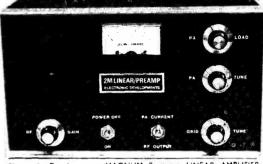
Electronic Developments MAGNUM 2 metre LINEAR AMPLIFIER. MICROWAVE MODULES, Rx Pre-amp, RF switched. Self contained power supply. Full input and output relay switching. Up to 100 watts SSB output. PRICE £105.00, post £1-00.
