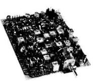
AT 222. A complete transmitter exciter unit for 144-146 NHz on AM or FM. VFO controlled or fixed channel operation. Complete with microphone pre-amp. speech processor including active audio filter. I watt output. FM. -25 watt AM. Output impedance 50-75 ohm adjustable. Frequency deviation 3-10 kHz adjustable.
