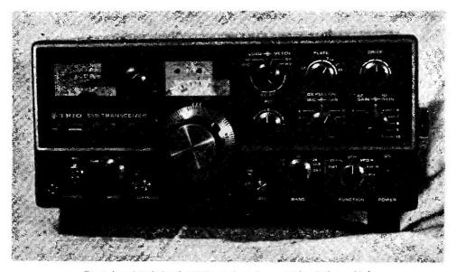
Front view of the Trio TS-520 Transceiver. A carrying handle is provided at the right-hand side of the cabinet, with some extra feet on the left panel drop, so that it can be carried and set down just like a brief-case.
