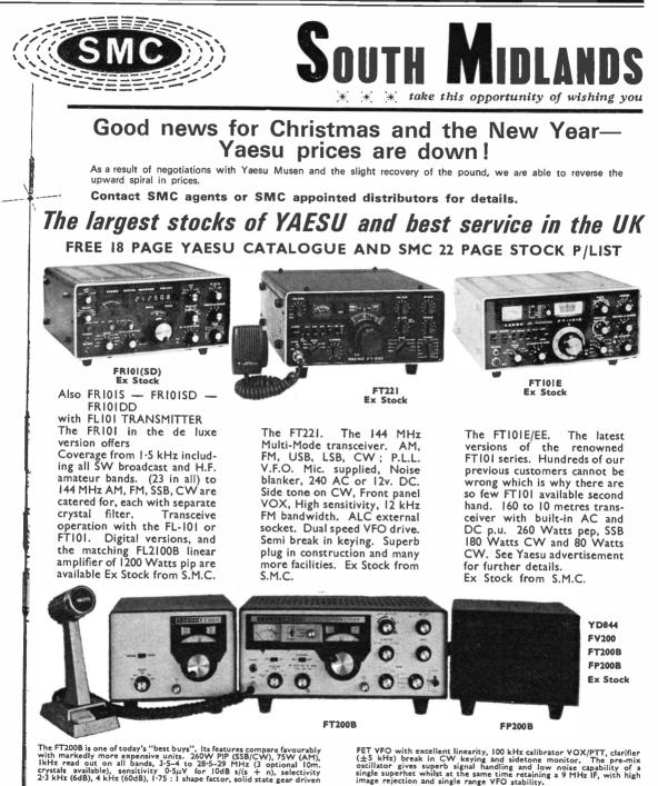
FET VFO with excellent linearity, 100 kHz calibrator VOX/PTT, clarifier  $(\pm 5 \text{ kHz})$  break in CW keying and sidetone monitor. The pre-mix oscillator gives superby signal handling and low noise capability of a single superhet whilst at the same time retaining a 9 MHz IF, with high image rejection and single range VFO stability.
